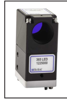
LED cube (bottom) and filter cube (top)
