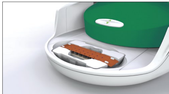
Fig. 2.5. Loaded DG8 cartridge placed in the QX200 droplet generator.
